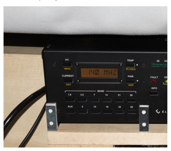
The amp sits on a shelf right on top of the inverter. With the bonding and a few ferrite cores, the noise is not too bad. There is way more RFI from every vehicle and power line around me. There does not seem to be any effect on vehicle or RV electrical systems.
