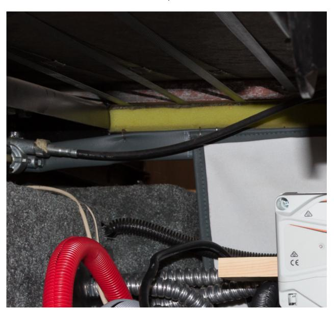
There is an Alpha Delta lightning arrestor and the DC power cables for the kX3, PX3 and antenna control feed to the right of the picture.
