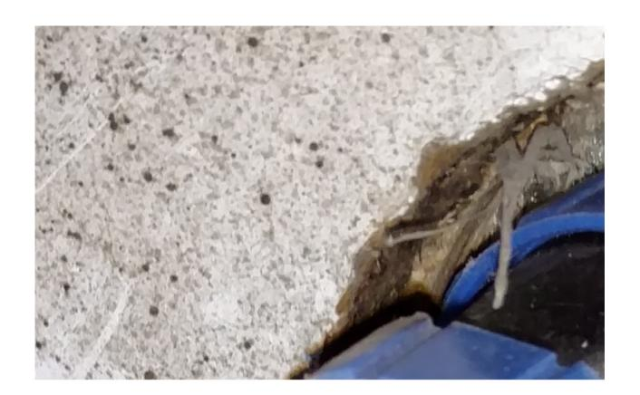
Inside the rear of the RV, the lines connect through the same plate the DC power cables from the house batteries to the 2 kW inverter go through, and are tied to a central ground point for all the equipment in the rear.
