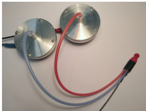
Figure 1 – Photograph of the sound reproduction system consisting of two DD45 earphone transducers (top left) coupled with the Etymotic ER-10B+ system (bottom right) via two tubes.
